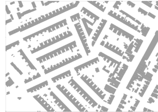
Figure ground plan of grid-iron terraces (above Figure 9) and medium intensity suburban development (below Figure 10) that illustrate the fine urban grain and consistent rhythm of building spacing and setbacks
