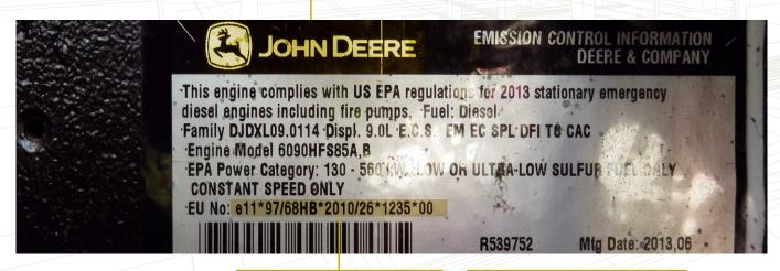
Type Approval Number: e11\*97/68HB\*2010/26\*1235\*00 Power output: Not shown, check external plates
